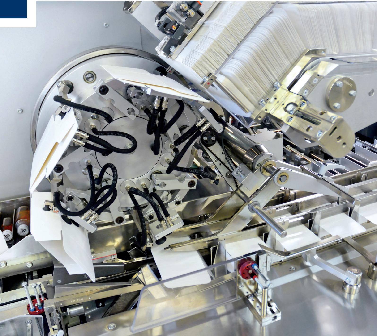
The operator side of the **HV** is perfectly linear and accessible, allowing carton magazine loading to be carried-out with convenience and with large carton storage capacity. This feature also gives the operator full vision and total control of all the functions carried-out on the machine.
